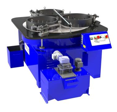
The Lapmaster Model 56 is equipped with a 1422mm diameter lap plate. This is manufactured from Grade 300 grey cast iron to ISO 185(2005). It consists of individual segments bolted to a support plate.
