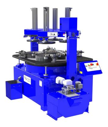
The Lapmaster Model 48 is equipped with a 48 inch (1219mm) diameter lap plate. This is manufactured from Grade 300 grey cast iron to ISO 185(2005). It consists of individual segments bolted to a support plate.
