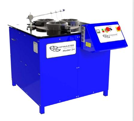
The Lapmaster Model 24 is the smallest floor standing lapping machine in the range and is ideal for engineering workshops, where flatness and finish are of prime importance. It is equipped with a 610mm diameter serrated lap plate, manufactured from Grade 300 grey cast iron to ISO 185(2005) as standard. Other plates can be supplied on request.
